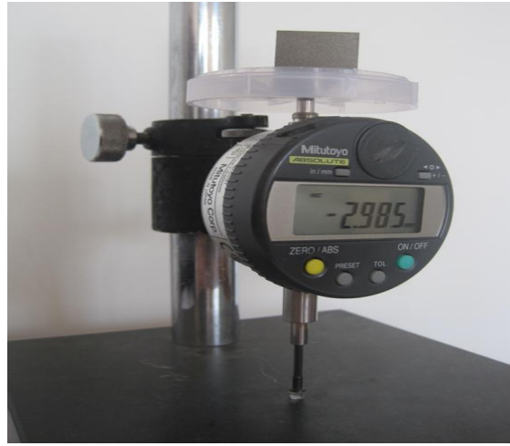
Figure 18 PDMS compression setup for measuring elastic modulus [2].
